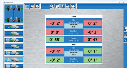
Simultaneously displaying the measured angles for each of the 4 wheels and proper zoom in the adjustment process
